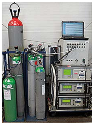
Figure 6. View of the mobile set of SIEMENS analysers used for exhaust gas composition testing Source: Own elaboration.
